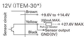
GND (Black) should be shared in case that power supply for sensor circuit (Brown) and that for sensor pull-up (Yellow) are separated.
