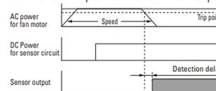
Example 3: When the DC power for sensor is first powered on, then the AC power for the fan is turned on
