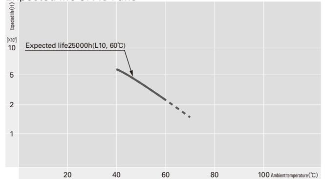
Rated voltage, continuously run in a free air state, survival rate of 90%
