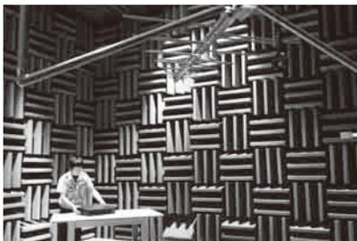
Acoustic radio wave anechoic chamber
