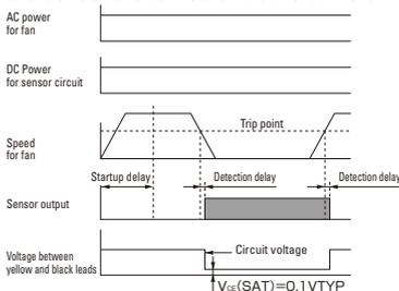
Example 2: When the AC power for the fan is turned on first, then the DC power for sensor is powered on
