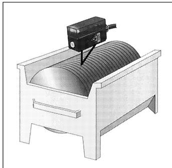
Detecting the presence/absence of an inserted part
