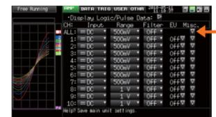
Parameters in AMP settings for 10 channels can be set at once using the ALL field.
