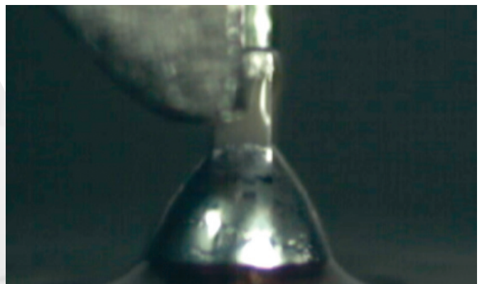
Figure 3 - 2.5mg pellet with 0201 resistor
