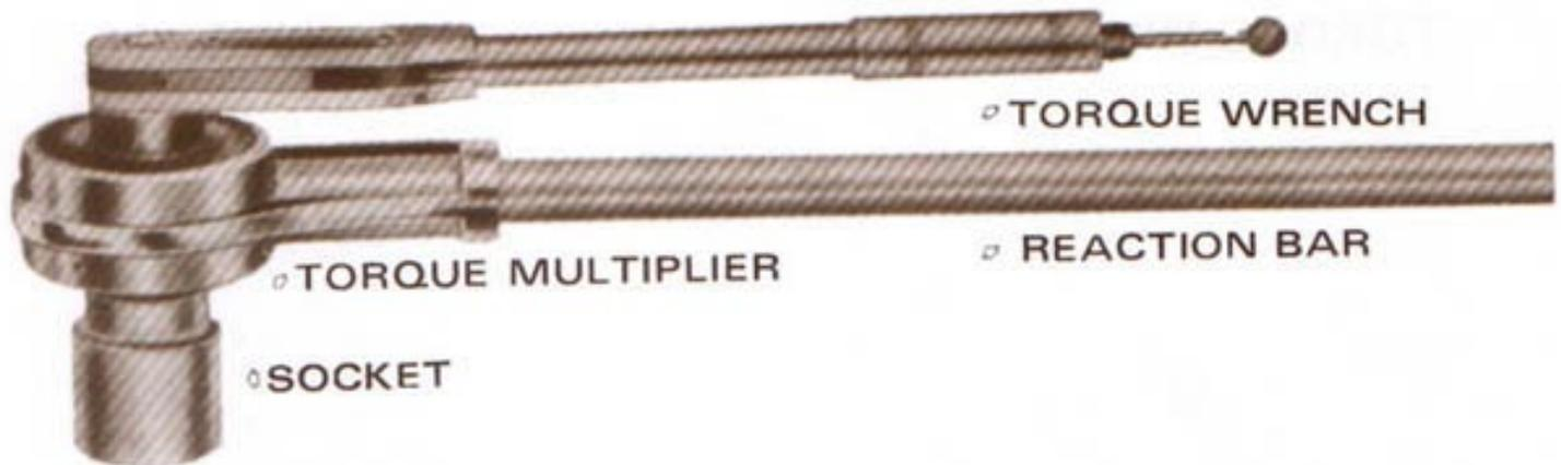
POWERMASTER TORQUE MULTIPLIERS are compact alloy steel, epicyclic gear units, designed for tightening and loosening of nuts and bolts and for providing very high torque economically.
