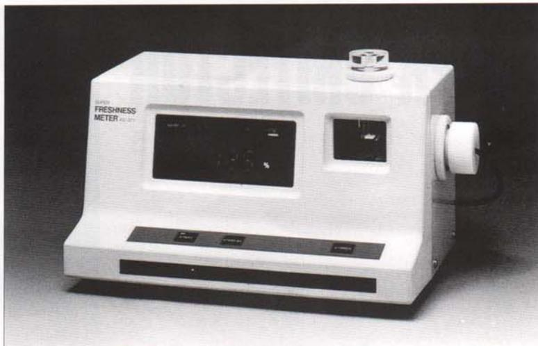
Rapid measurement of "K value," the decisive factor in freshness, is now possible. Reliable instrumentation is also available, eliminating virtually all dependence on skill or experience.
