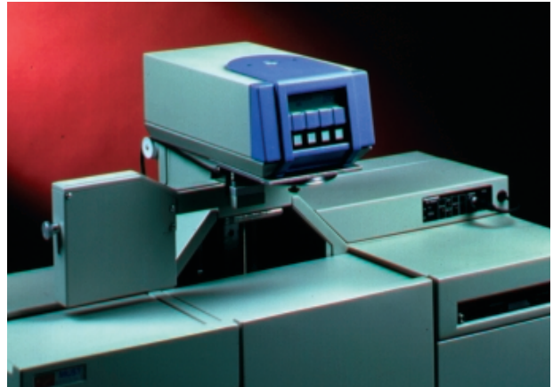
The Video Alignment System, showing the swing-arm containing the video lens and camera head (front left of photo), and the power supply/camera box (back right of photo)
