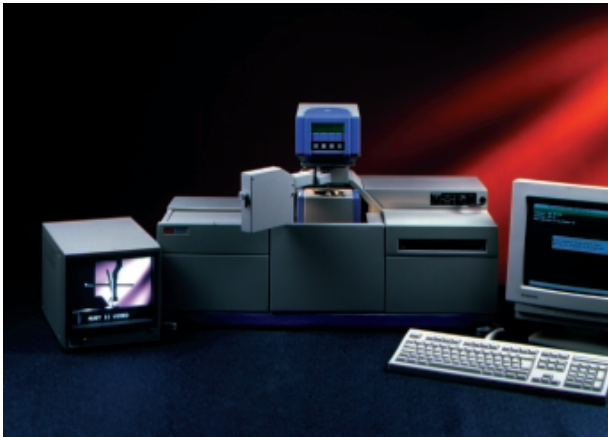
The MUST System II with Video Alignment Option, showing the video alignment monitor (left of photo), swing-arm containing the video lens and camera head, and the power supply/camera box
