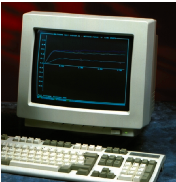
Typical force vs time curve from microwetting balance test
