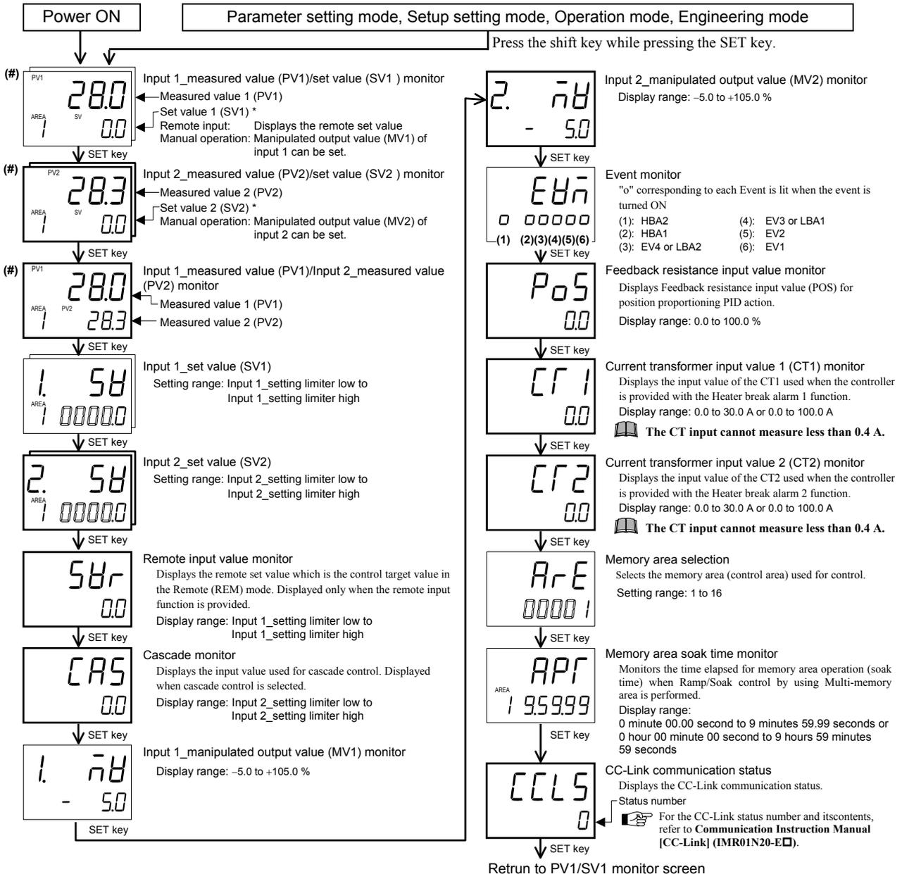
\* With the Setting change rate limiter when the set value is changed, the displayed set value changes according to the ramp-up/down rate.
