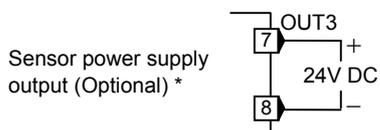
\* Output 3 can be used as a power supply output (optional) for the transmitter (pressure sensor, temperature sensor, etc).
