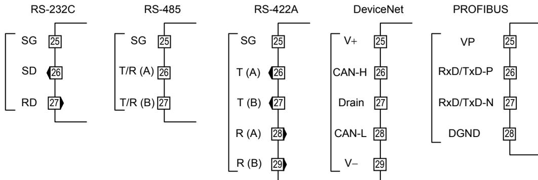
Example 1: Connection to the RS-232C port of the host computer (master)
