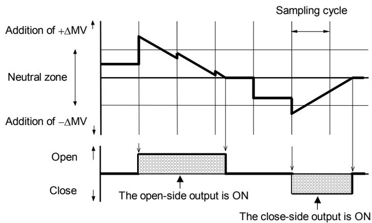
The controller does not output the  $\Delta MV$  to a control motor when the PID computed output value is within the neutral zone.
